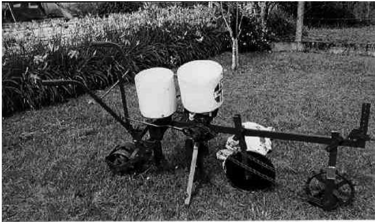
Photo 4. Animal-drawn no-till planter with seed and fertilizer tanks (Paraná, Brazil)
